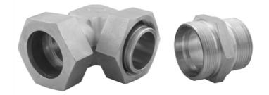
Adjustable elbow coupling made of stainless steel DIN 2353, EN ISO 8341-1
