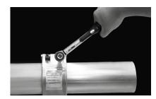
Do not rotate the pipe coupling on the pipe as long as the anchor teeth are engaged (Axilock only).
