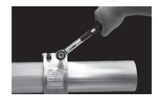
· Do not rotate the pipe coupling on the pipe as long as the anchor teeth are engaged (Axilock only).
